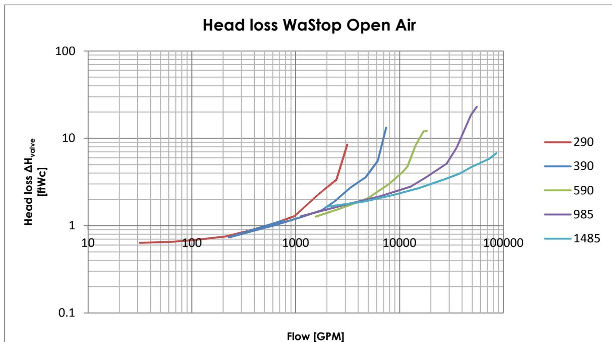
Fig. 5 Open Air Head loss (US)
