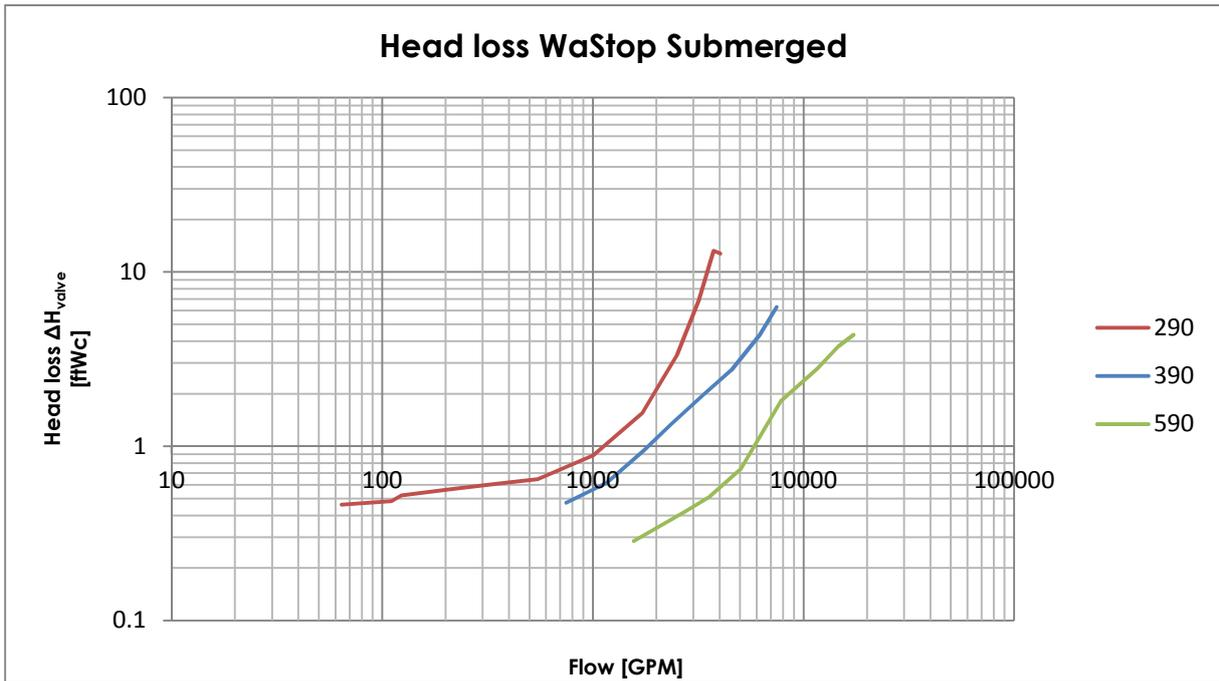
Fig. 6 Submerged head loss (US)
