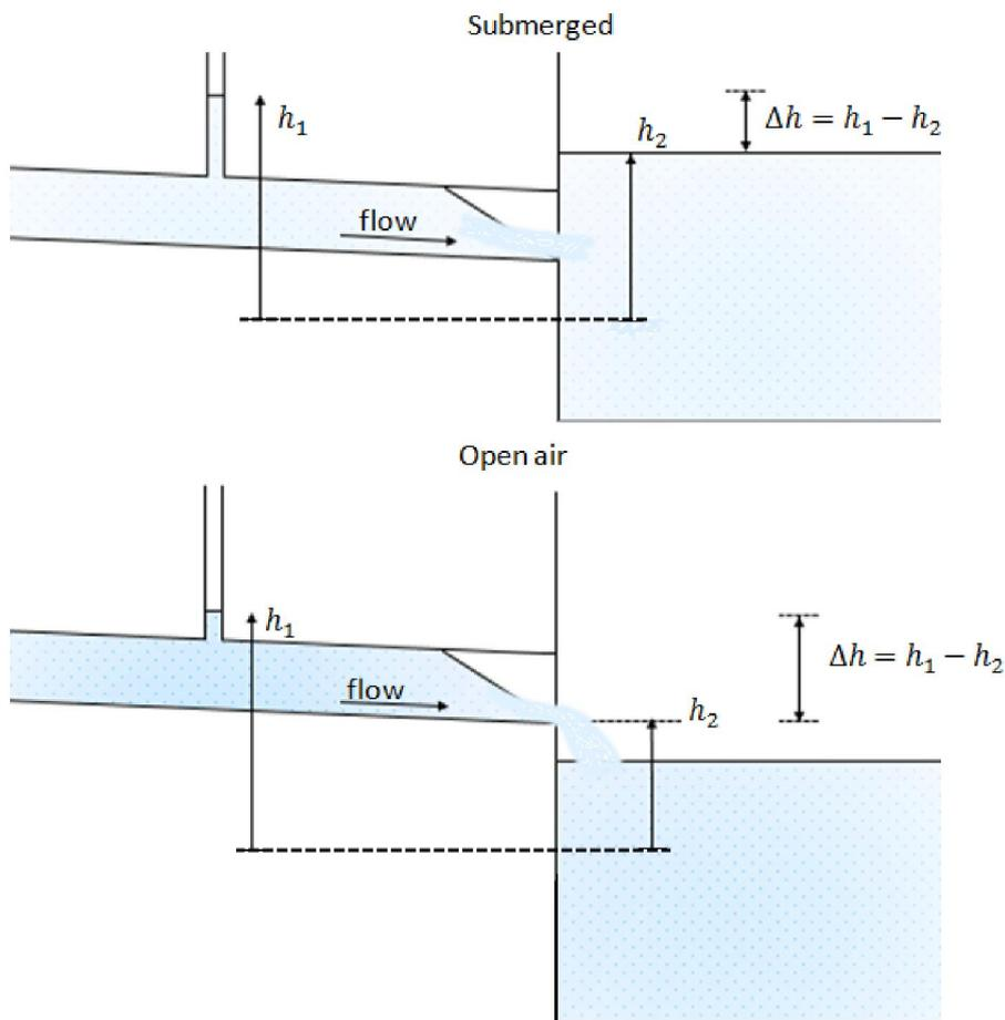
Fig. 1 Opening pressure and head loss definition.
