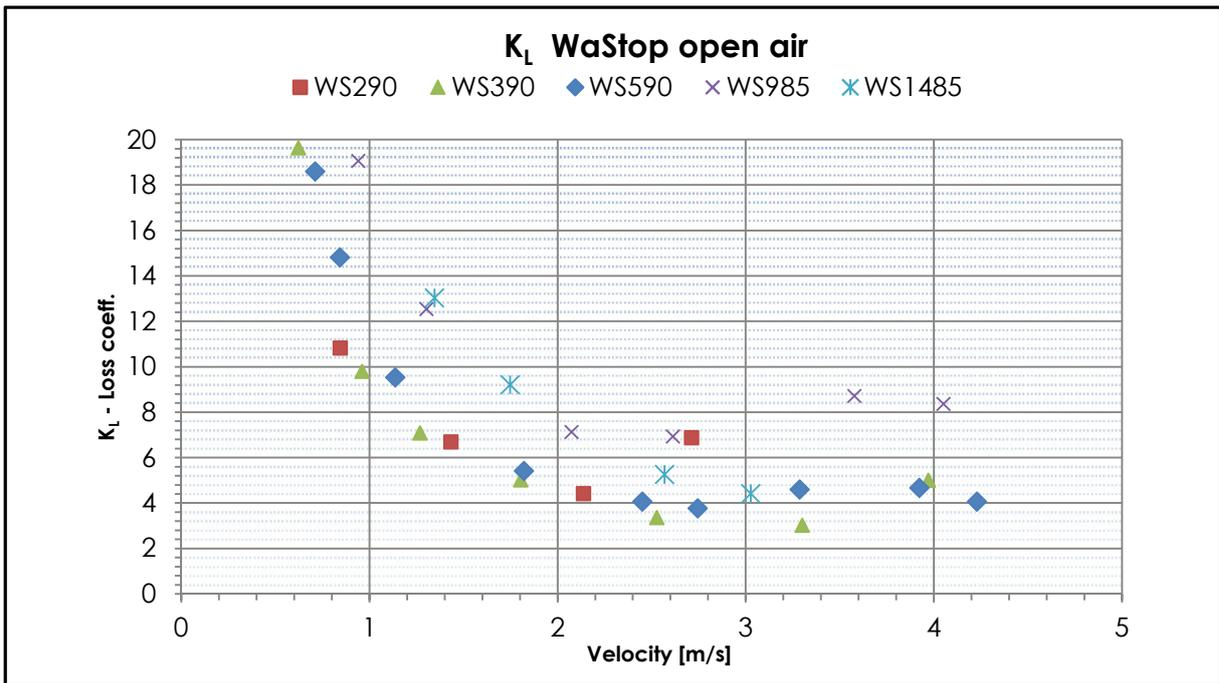
Fig. 7 K<sub>L</sub> WaStop open air
